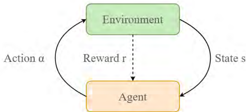
Figure 3.1: Interaction Loop between Environment and Agent in RL.
